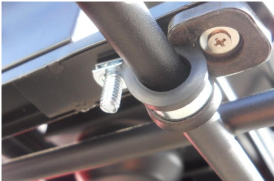
Close up of loop clamp from below the grill.
